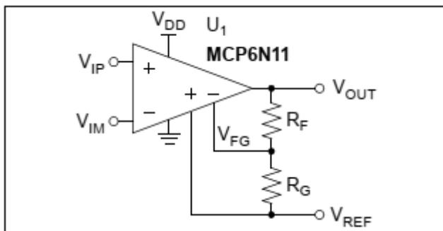
$$V_{OUT} \approx G_{DM} \times (V_{MES} - V_{REF})$$
